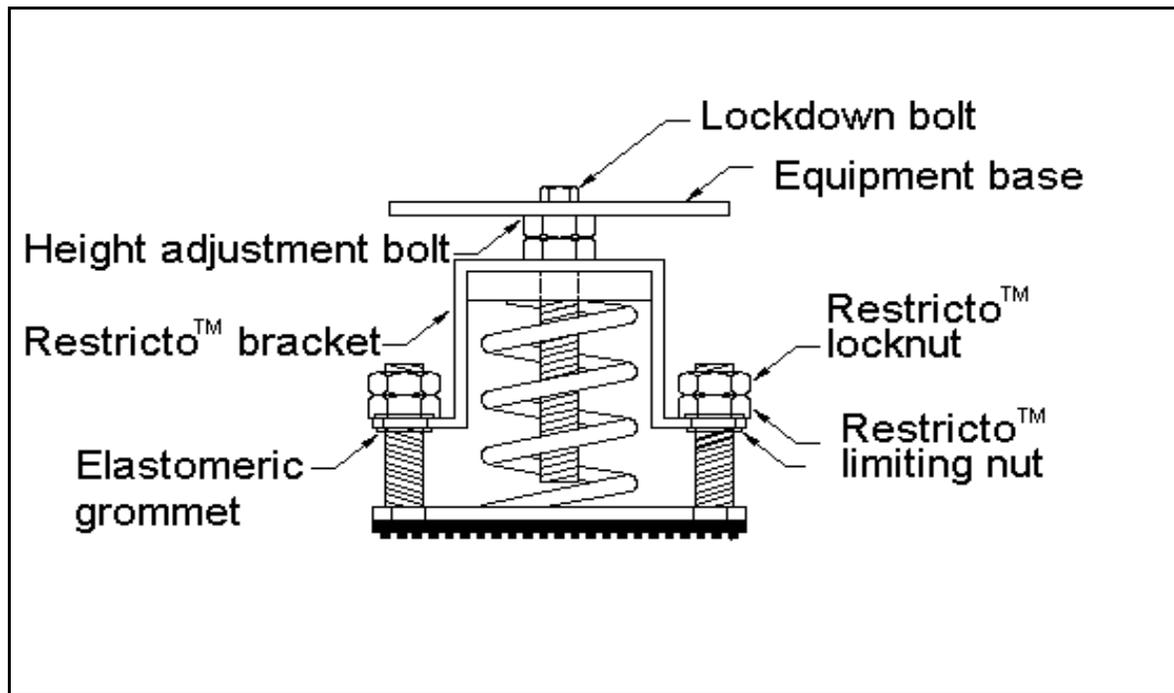
\* Figure shown is single spring isolator. Installation instructions remain the same for multiple spring isolators.
