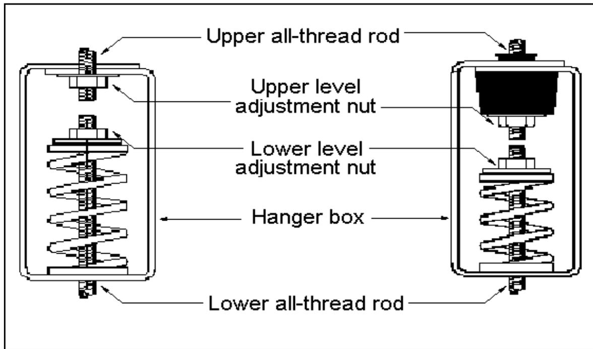
\* All-thread rods, level adjustment nuts, upper level adjustment washer by others.
