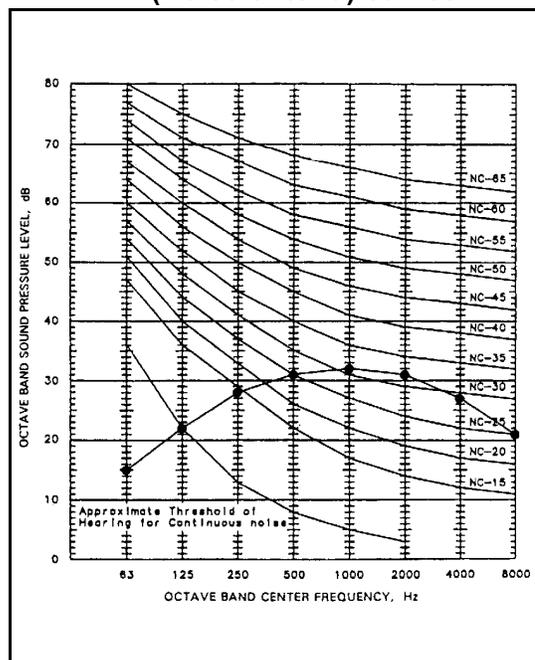
Based on above data, equipment noise levels, and STC rating of existing structural slab, a determination has to be made whether any further transmission loss is required between the mechanical and receiver rooms. If so, a **VIMCO** floating floor offers a possible solution.
